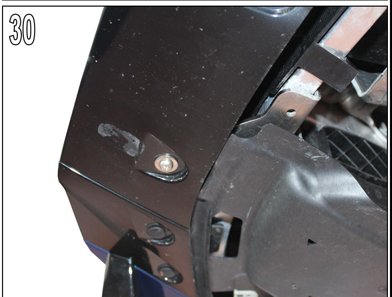
Fig. 30 Align the AC Schnitzer holder with the aluminium cross member on the outside. The rivet nut on the holder must be aligned with the hole in the standard front skirt.
