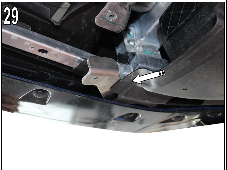
Fig. 29 Insert the AC Schnitzer holder outer between the standard front skirt and the aluminium cross member.
